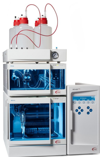
Figure 1. ALEXYS Carbohydrate Analyzer—isocratic, consisting of the ET 210 eluent tray (for \text{N}_2 blanketing), a P 6.1L pump with solvent selection valve and dual channel degasser, AS 6.1L autosampler and DECADE Elite electrochemical detector.
